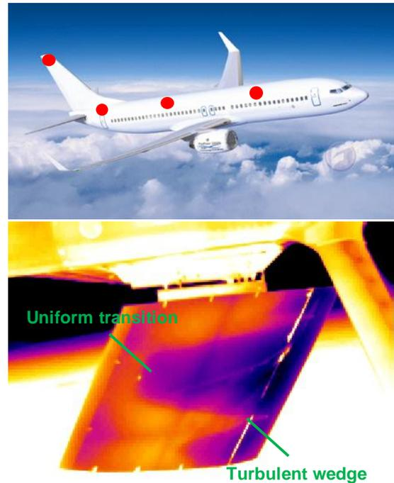
Figure 3. Possible installation of IR cameras (top) and a notional example of IR image (bottom; flow right to left)
