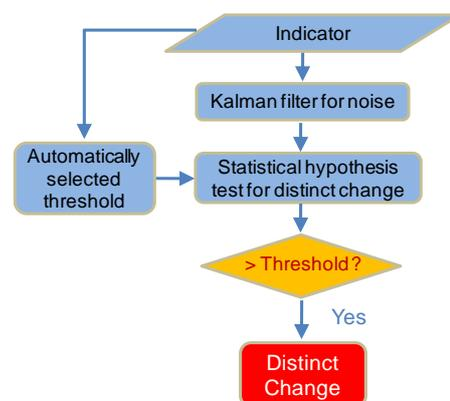
Figure 6. Overall logic flow for the detection module.
