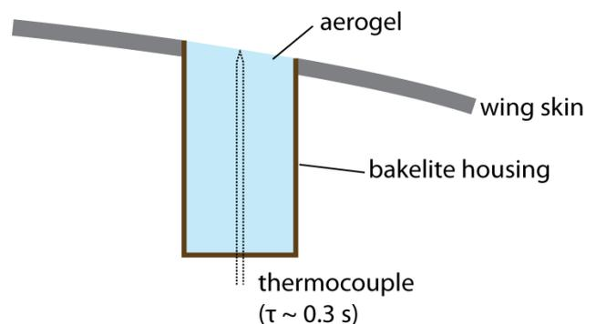
Figure 4. Insulated thermocouple sensor concept. The thermocouple is insulated from the wing skin in order to measure freestream adiabatic recovery temperature.
